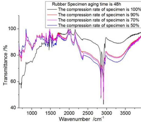
**Figure 3. Infrared spectroscopy analysis of rubber aging.**
