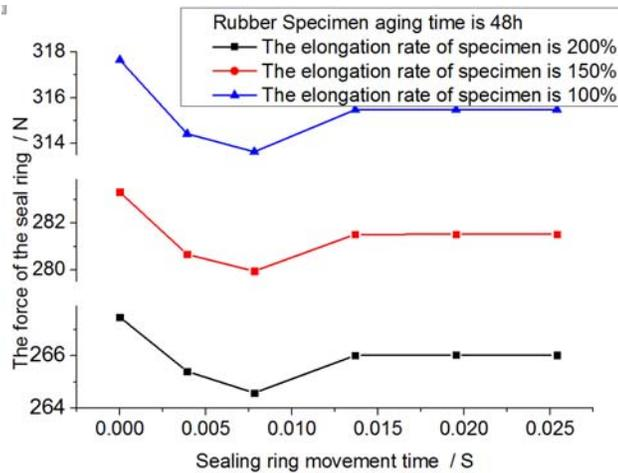
Figure 6. Normal forces in dynamic friction.
