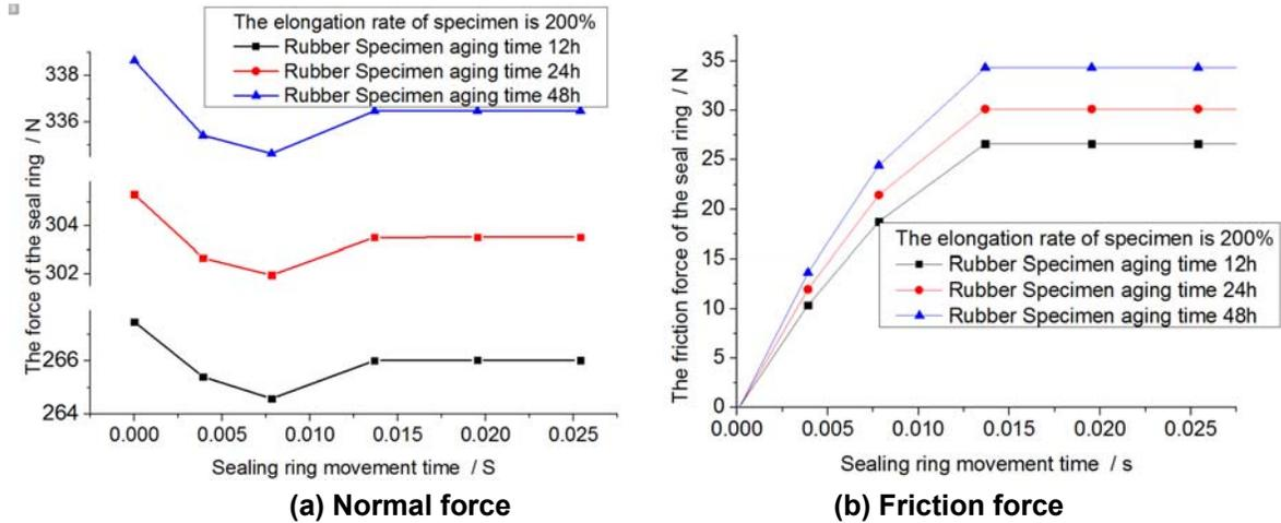
Figure 5. Effect of aging on the contact forces.
