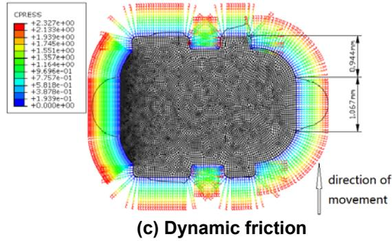
Figure 4. Dynamic friction of the seal ring.
